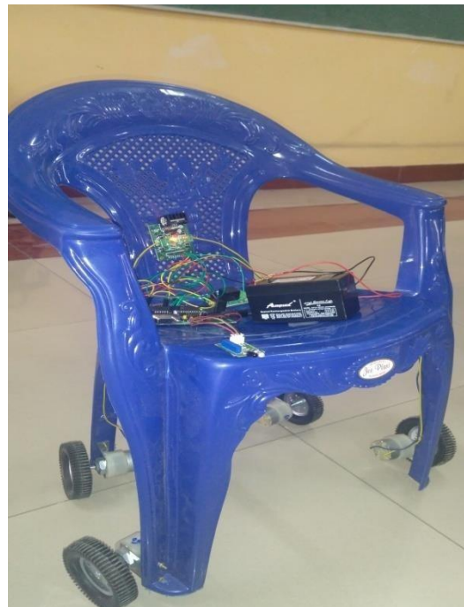
Fig d): Interfacing of Android Smart phone and the wheelchair.
