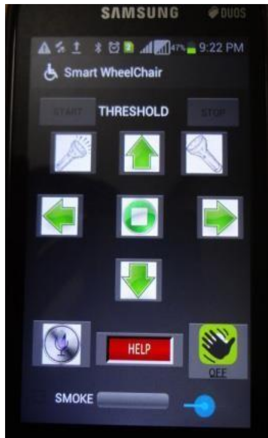
Fig. e) shows the Android application for the operation of Wheelchair.
